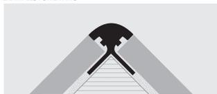
**PROKERLAM JOLLY** is a quarter-circle rounded bead profile in anodized and polished aluminium suitable to protect the external corners of coverings with low thickness. It can be used like connection profile between step tread and riser of stairs coated with ceramic and mosaic with low thickness. Its particular section and the availability in three different finishes make **PROKERLAM JOLLY** a much sought-after profile that allows a workmanlike application even with low thickness coverings.
